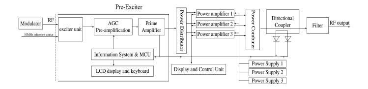
PS: This diagram is a reference for 800W and 1000W transmitter. For 1200W transmitter, there are 4 power amplifiers and 4 power supplier included.
