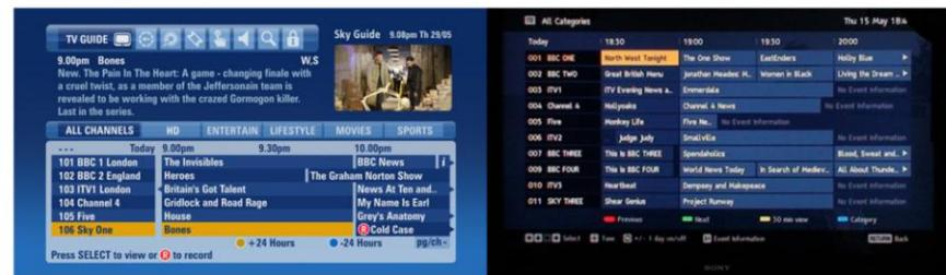
Dexin EPG is a fully-complying DVB standard system for uniform distribution and collaboration of DTV broadcasting network resources. It supports PSI/SI standard tables, standard descriptors, private descriptors, private application data generation and scheduling for broadcasting.
